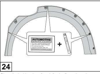
Clean the inside edge of each fender flare where the rubber extrusion will adhere. Use the provided alcohol wipes. Once dry apply primer to the contact area of the extrusion adhesive tape and allow to flash off.
