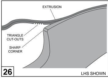
The extrusion has multiple triangles out of the extrusion where it meets the sharp corners as shown.
