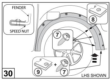
Attach the rear part of the rear fender flare with (3) Hex head screws and factory plastic nuts. Secure the rear lower part with one hex head screw and Speed nuts as shown.
