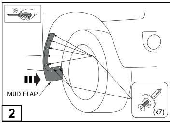
Remove the mud flaps by removing the (7) scrivets from inside the wheel arch as shown.
