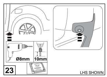
Carefully drill through centre of rivet holding the liner with a Ø8mm drill bit & and 10mm drill stop as shown. Carefully remove the reminder of the rivet using needle nose pliers. Apply rust inhibitor to the holes.
