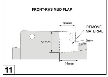
Measure and mark Mud Flap area to be removed, as shown. Using tin snips remove the white area. Repeat for the LHS Mud Flap. Remove all the masking tape.
