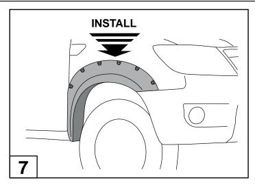
Fit the fender flare to the vehicle in the uppermost vertical position, before final fixings and tape application is completed as shown.
