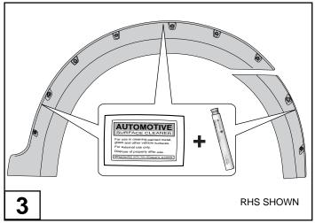
Clean the inside edge of each fender flare where the rubber extrusion will adhere. Use the provided alcohol wipes. Once dry apply primer to the contact area of the extrusion adhesive tape and allow to flash off.
