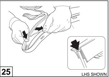
Pulling at right angles to the extrusion, remove the liner from the extrusion in small portions and apply thumb pressure to ensure that it adheres to the Fender Flares. Trim any unnecessary extrusion and discard.
