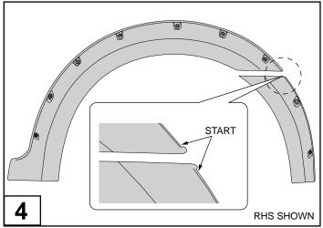
Remove approximately 50mm of the protective liner from the extrusion. Fit the extrusion to the Fender Flare along the edge that comes in contact with the vehicle's body panel. **NOTE:** Start applying the extrusion from area shown above.
