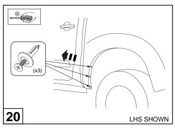
Remove the (3) scrivets from inside the rear wheel arch as shown.
