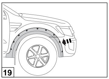
Fit the bumper flare to the vehicle as shown.
