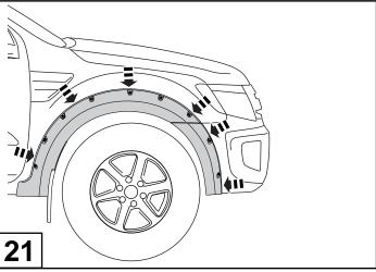
Ensure that flares are aligned. Remove the tape liner. Apply firm pressure on the flare to ensure the tape is contacting the vehicle surface around the full perimeter of the flares.
