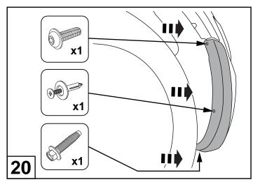
Secure the flare using previously removed screw and scrivet as shown.
